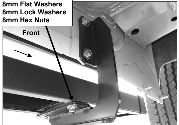
(Fig 8) Driver/left front mounting Bracket installed
