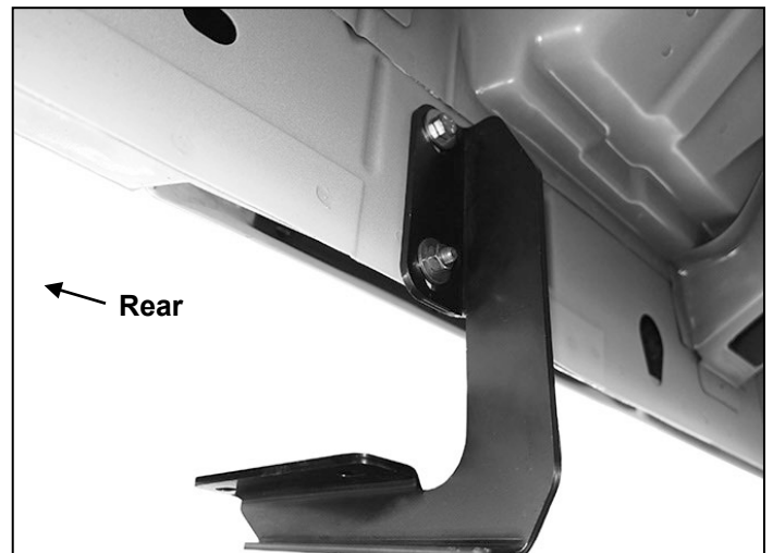
(Fig 4) Driver/left rear Mounting Bracket installed
